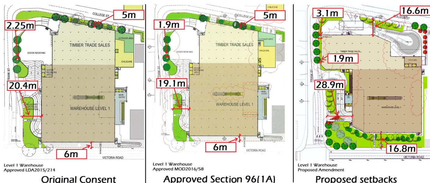
Figure 9: Changes to building setbacks
